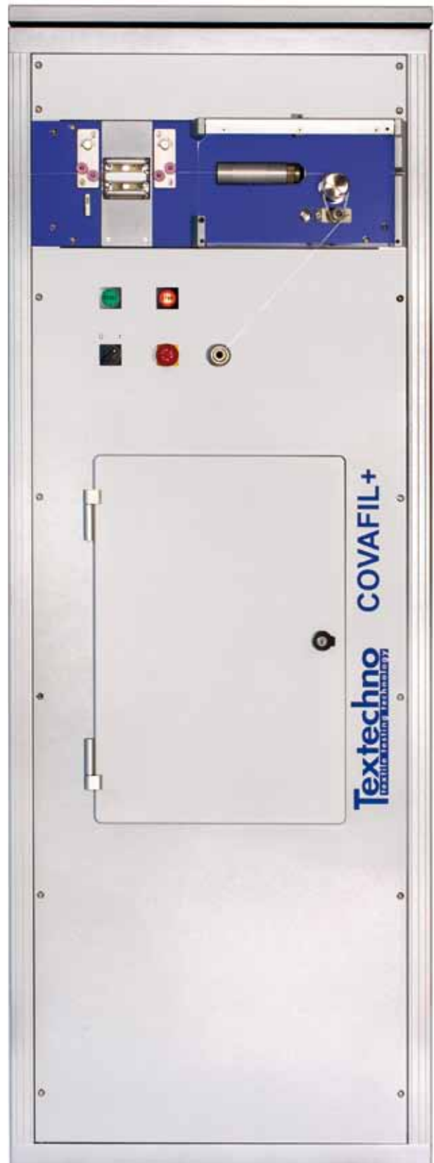
COVAFIL+ Capacitive evenness tester for filament yarn
